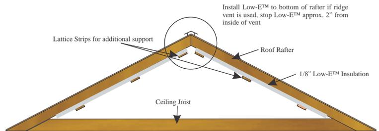
Note: If pre-manufactured truss assembly is used, retro fit between trusses with Low-E™ 16" / 24" Tab Material to avoid bracing cuts.
