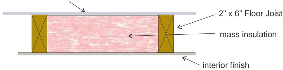
Low-E™ Attic Floor can be rolled out over existing mass insulation. The product is perforated and will not trap moisture. Low-E™ Attic Floor can be stapled with 1/2" staples every 6". Since it is not a vapor barrier taping of seams is optional.
